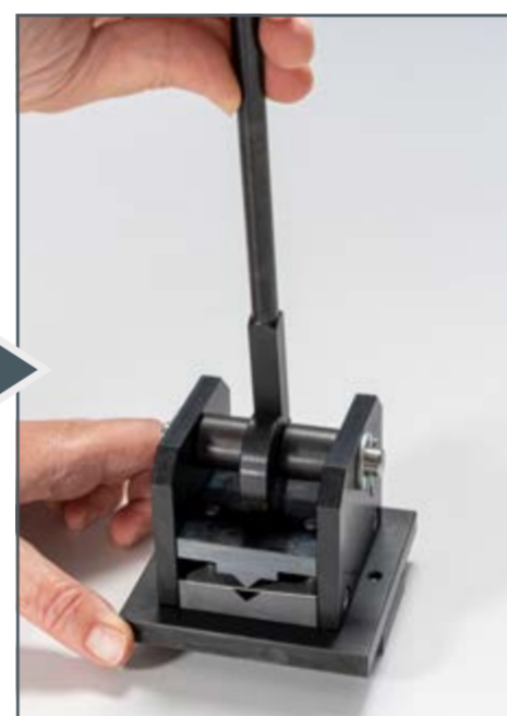
Forming the workpiece with the bending press from TZ 200.01
