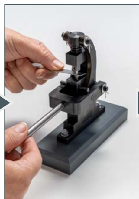
Punching holes with the lever press from TZ 300
