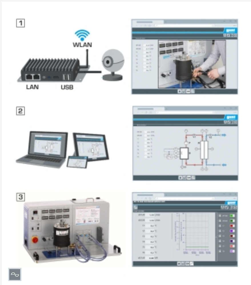
Exemplary experimental setup: 1 GU 100 Web Access Box with live image transmission, 2 various end devices with access to software via web browser, 3 experimental unit with measurement data acquisition
