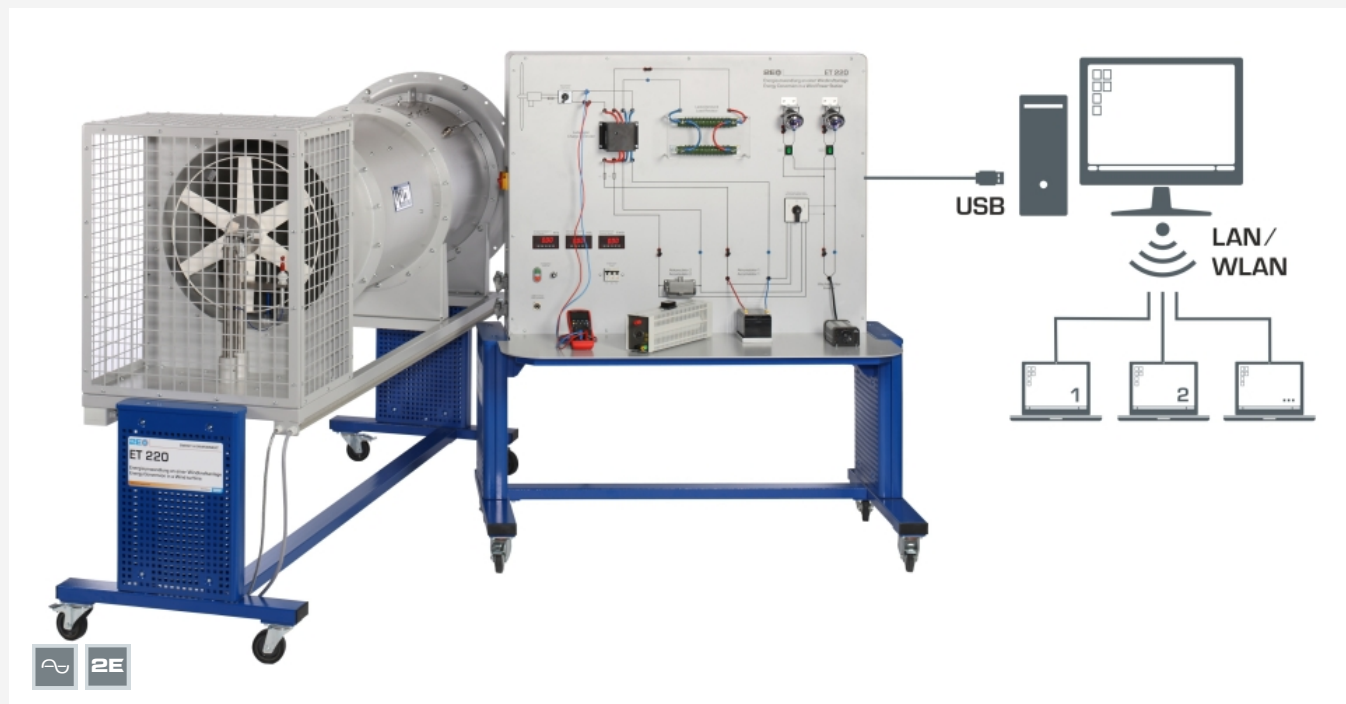
Network capable GUNT software for data acquisition: observation, acquisition, analysis of the experiments at any number of workstations via the customer's own LAN/WLAN network.
