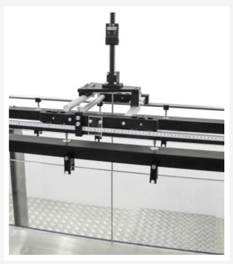
The illustration shows a similar water level including digital display mounted on an instrument carrier.
