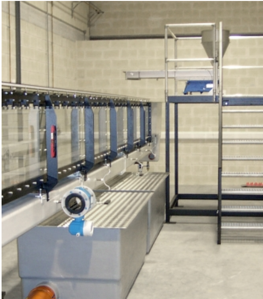
The illustration shows the sediment feeder on the platform.
