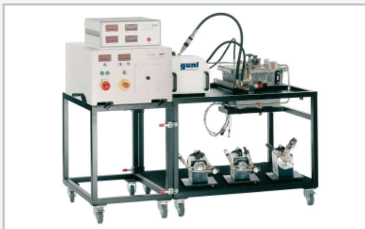
Functional experimental setup: drive unit HM 365 (left), HM 365.20 with pump under investigation (right)
