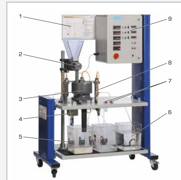
1 process schematic, 2 spiral conveyor for extraction material, 3 revolving extractor, 4 revolving extractor drive unit, 5 pump (behind the tanks), 6 tank, 7 mode selector valves, 8 heater and solvent feed, 9 switch cabinet with controls
