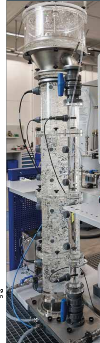
Various distributors for aerating the reactor
