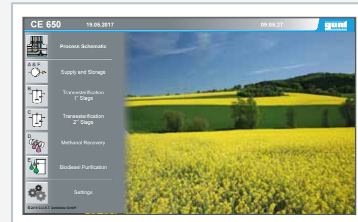
Start screen of the PLC for operation of the experimental plant
