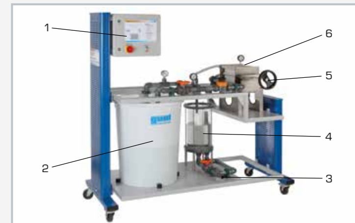
1 switch box with controls, 2 suspension tank, 3 filtrate tank outlet and overflow, 4 filtrate tank, 5 spindle, 6 plate and frame filter press
