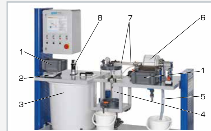
1 filter cake collector tank, 2 balance, 3 suspension storage tank, 4 filtrate vacuum tank, 5 overflow/outlet, 6 drum cell filter, 7 vacuum supply, 8 stirrer
