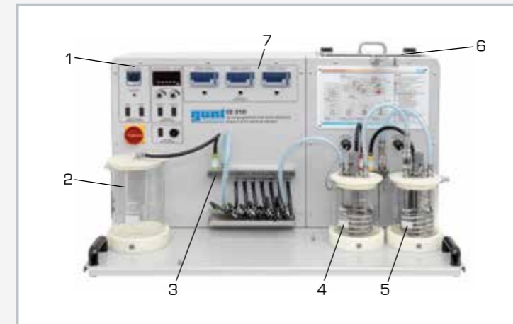
1 displays and controls, 2 product tank, 3 connection block, 4 and 5 tanks for reactants, 6 water tank, 7 display of conductivity and temperature
