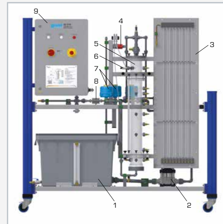
1 treated water tank, 2 backwash pump, 3 manometer panel, 4 differential pressure sensor, 5 filter, 6 system pressure sensor, 7 ball valve with motor, 8 flow rate sensor, 9 switch cabinet
