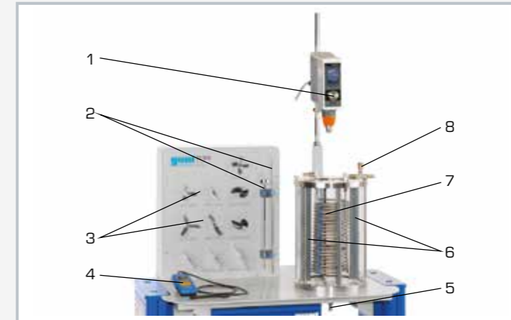
1 stirring machine with speed and torque indicator, 2 turbine stirrer and threaded shaft for stirring heads, 3 stirrer elements, 4 conductivity meter, 5 outlet, 6 flow impeder, 7 coiled tube, 8 shut-off valve for coiled tube
