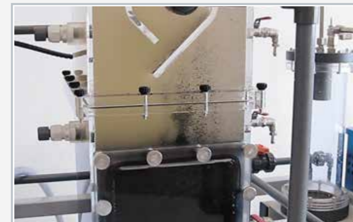
UASB reactor during experimental operation
