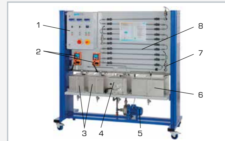
1 switch cabinet, 2 reactant pumps with volumetric flow rate measurement, 3 reactant tank, 4 hot water tank, 5 pump, 6 product tank, 7 measurement of temperature and electrical conductivity, 8 tubular reactor with 10 sections
