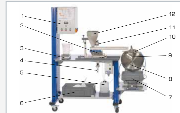
1 switch cabinet, 2 solid material metering device, 3 balance, 4 pressure reducing valve, 5 granulating liquid tank, 6 solids tank, 7 agglomerate tank, 8 dish granulator, 9 scraper, 10 two-component nozzle, 11 vibrator, 12 solids silo
