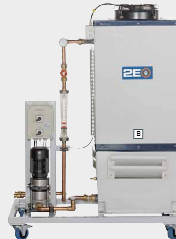
Wet cooling tower
