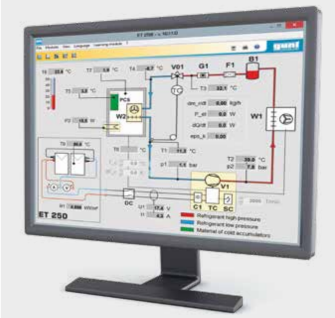
GUNT software for controlling the device and for measurement data acquisition via PC
