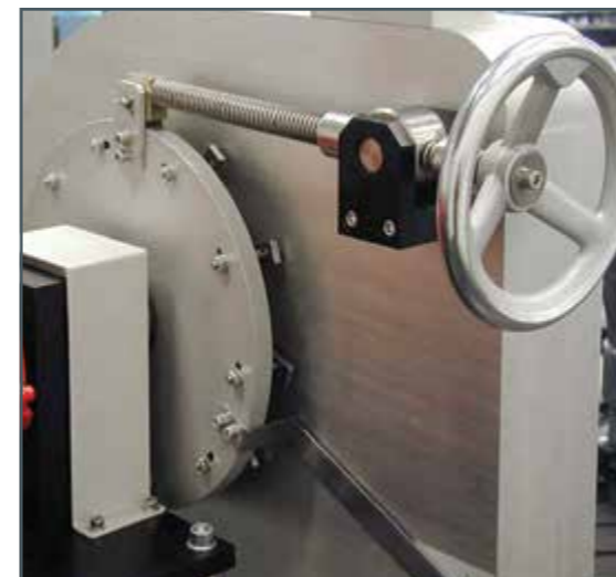
You can easily study the behaviour of the turbine with different distributor positions.
