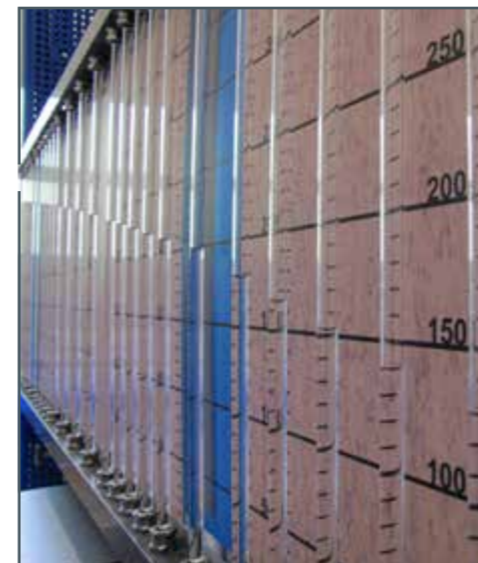
Manometer panel on the sand bed
