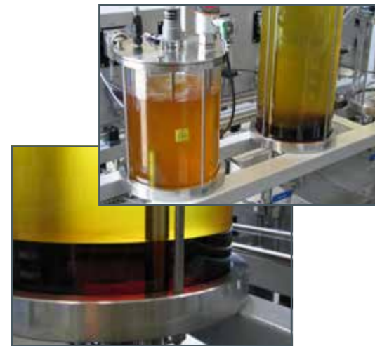
Transparent tanks allow continuous observation of reactions and separation processes.
