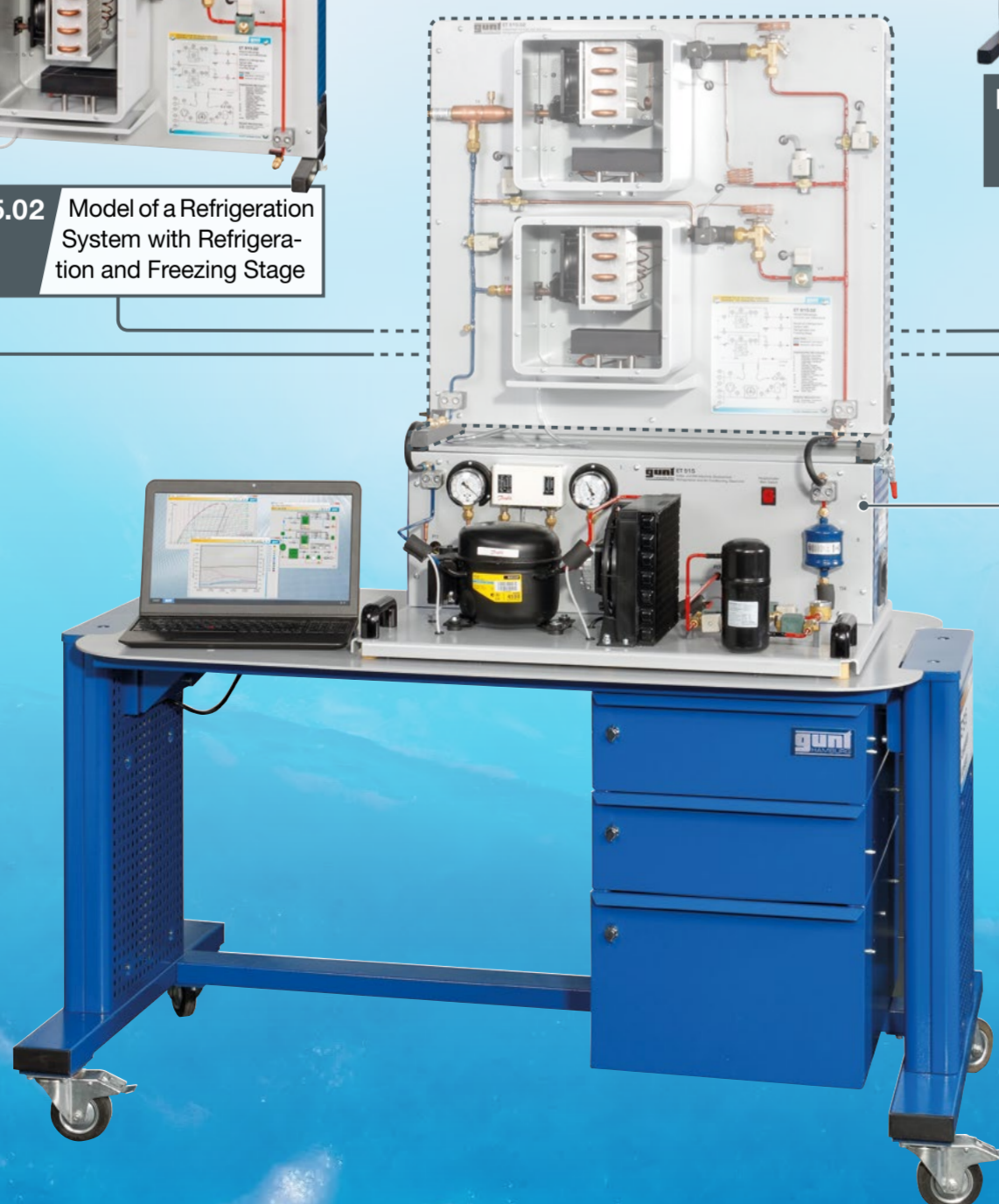
The ET 915 base unit contains the main compressor and condenser components
