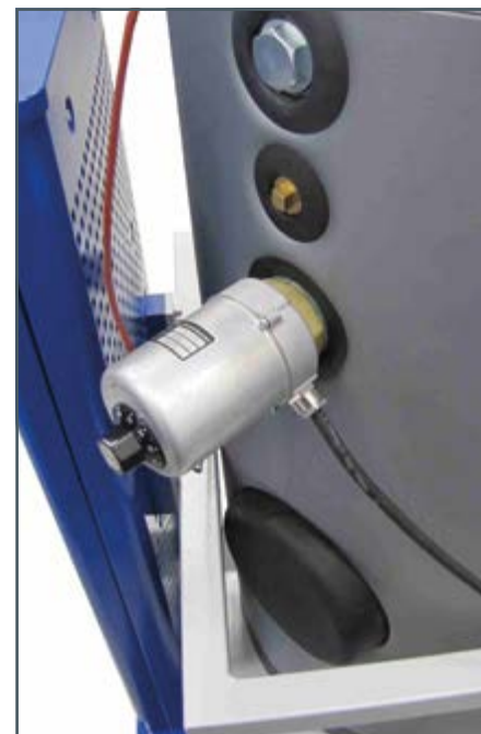
The storage tank is emptied in preparation for the experiment. The auxiliary heater can easily be inserted subsequently in just a few steps.
